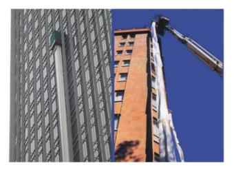
Called the Ingstrom Escape Chute (R), the technology has been developed by Mobiltex Evacuation Systems, a Swedish company. Is the technology new? No. On its website, Mobiltex describes it as "standard rescue equipment used by fire brigades worldwide for high rise rescue operations."
